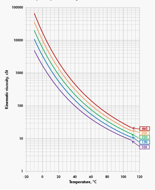
Viscosity - Temperature Diagram for Shell Morlina S3 BA
